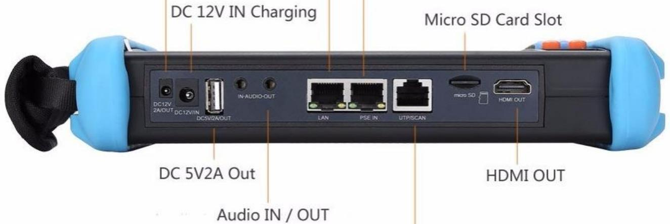
Test Interface of Network Connecting Cable Sorting /Line Hunting Test Interface
